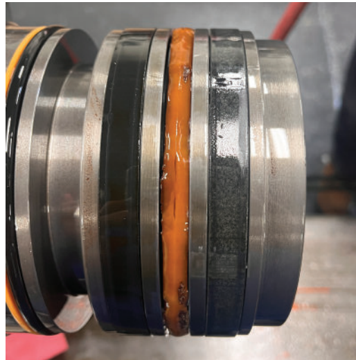
» This is an example of piston seal failure due to heat.
