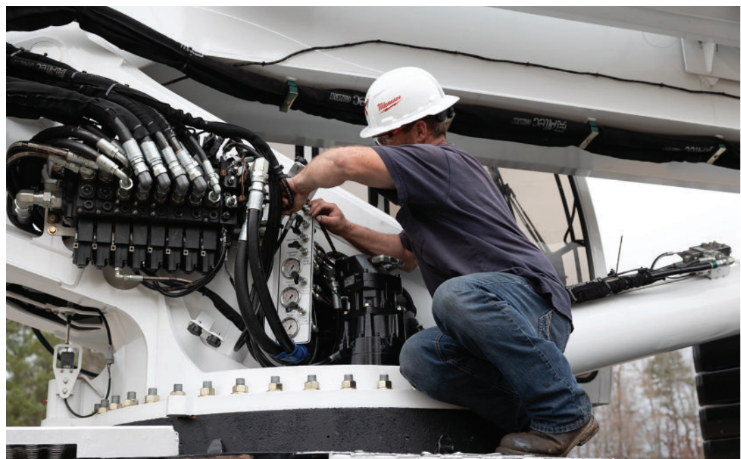
» Hydraulics don’t fail all at once, and routine checks can help fleets catch wear and contamination before they lead to costly downtime.
